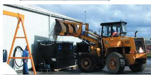
Easy filling of NaCl (salt): The mixing vessel construction allows filling of dry material by means of a
