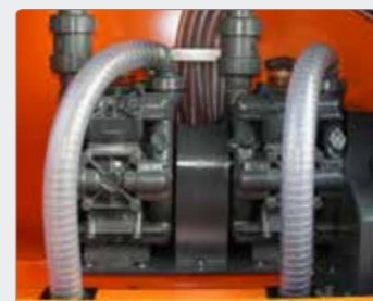
Logically built liquid system featuring diaphragm pump.
