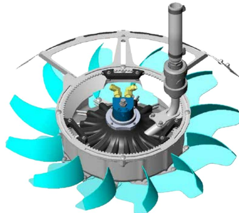
By means of the centrifugal force the specially designed mixing disc ensures that the salt grains and the liquid are mixed in a rotational motion inside the mixing chamber. In this way an optimal prewetting of each individual grain of salt and thereby a good adhesion to the road surface is ensured. Subsequently the best result when spreading prewetted salt (30% prewetting) is achieved.
