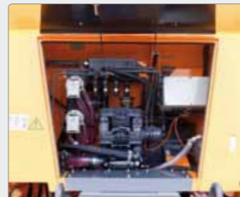
All vital components located together in an enclosed machine house, which offers protection against moisture and salt dust. The design increases user friendliness.
