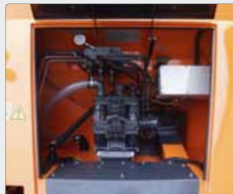
All vital components located together in an enclosed machine room, which offers protection against salt dust. Furthermore, the design has focus on increased user friendliness for drivers and service staff.
