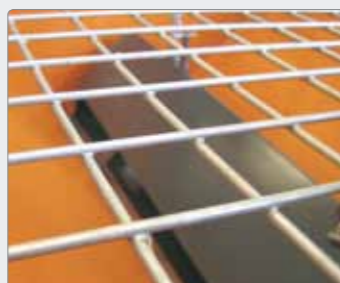
Relief plate minimizing the weight of the material on the conveyor belt (option)
