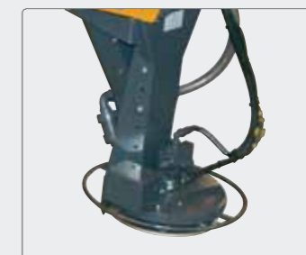
Stainless steel spreading disc and feed funnel
